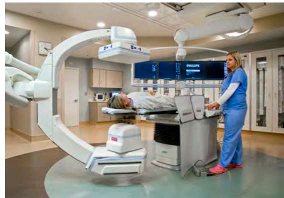
The new C-arm provides surgeons with immediate soft tissue images and real time 3-D viewing while operating.
